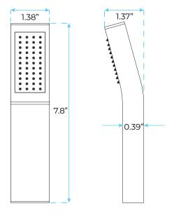
The minimum required water pressure is 0.05 MPa (0.5 bar). Flow rate 2.5 GPM (9.5 LPM).
